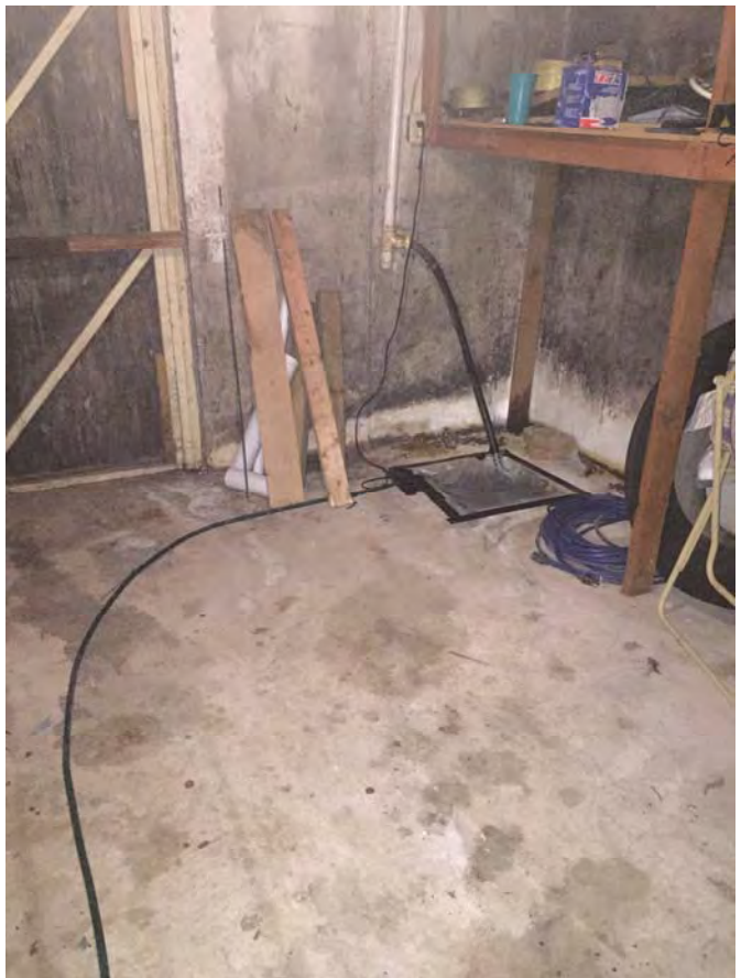
Sump hole was sealed off from the room using plastic sheeting and tape approximately 48 hrs prior to collecting headspace air and water samples.
