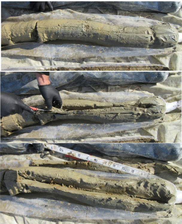
Figure 4-3. Examples of wedge sampling.
