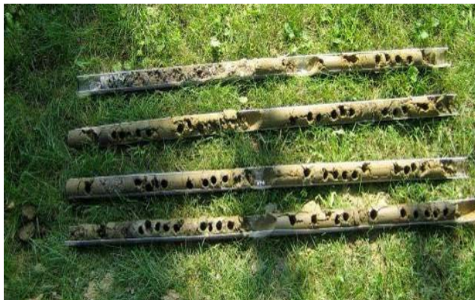
Figure 4-4. Examples of plug sampling.
